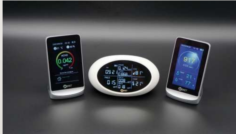
f) Air quality monitors Dust, VOC, CO 2 , temperature, humidity
