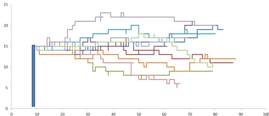
Figure 2 - Variants of calculating the possible trajectories of ten gas particles take in a turbulent flow ( $p_{+x} = 0.7, p_{-x} = p_{+y} = p_{-y} = 0.1$  (10x100 steps))
