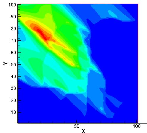
Figure 7 - The spread of harmful gas impurities from the linear source at a wind speed of 5 m / s in the northwest direction
