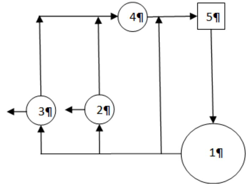
Diagram of air conditioning systems for drying fish: 1 - fish drying chamber, 2 - air cooler of the refrigerating machine, 3 - air cooler of the heat pump, 4 - condenser of the heat pump, 5 - circulation fan
